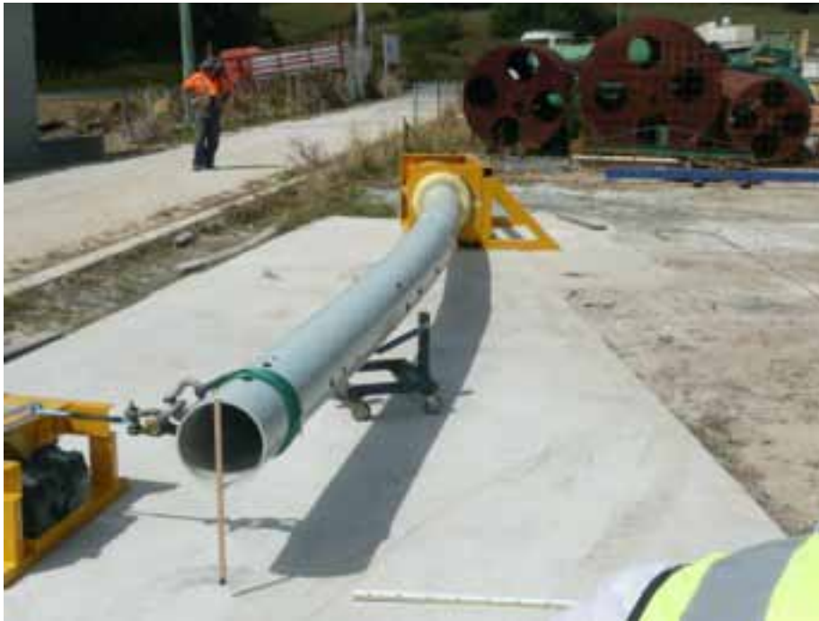
Fig 4. - Pole at 25kN Tip Load
